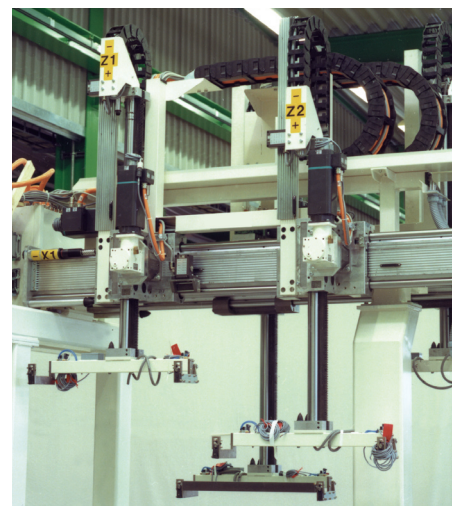
Dos ejes pick and place robot
